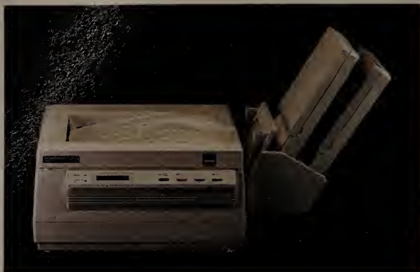
The MT906's Jade controller uses its own processor to describe images as quickly as it prints text, giving the laser effective throughput far beyond the TEC engine's 6-page-per-minute rating.
